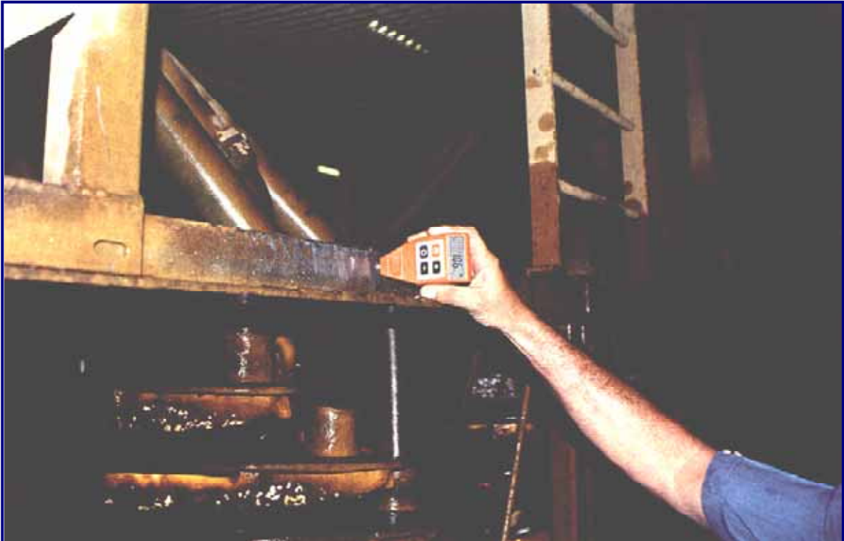
Site CRL2 (b) – 10mm thick ANGLE section coating thickness reading.
