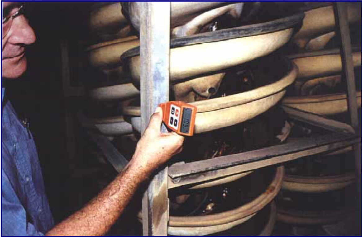
Site CRL3 (a) – 4.0mm thick RHS section coating thickness reading.
