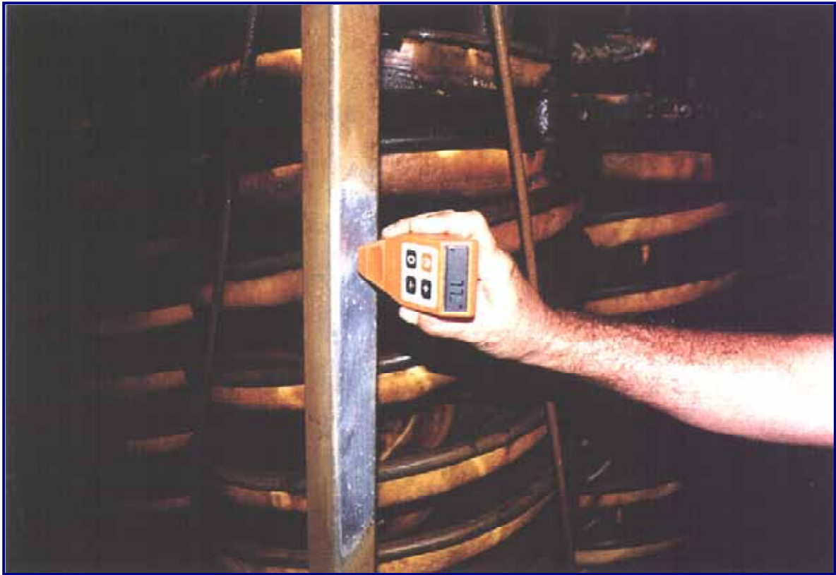
Site CRL2 (b) – 10mm thick ANGLE section coating thickness reading.
