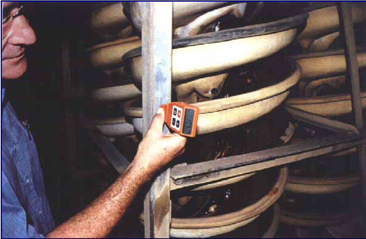
Site CRL3 (a) – 4.0mm thick RHS section coating thickness reading.
