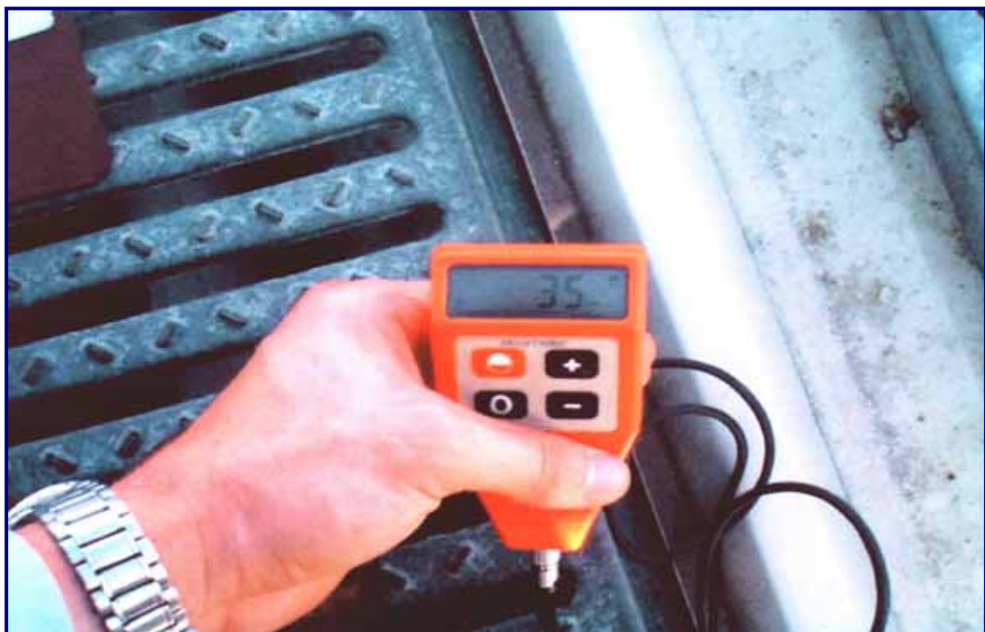
Deception Bay Shopping Centre – Bottom Lip Micron Thickness
